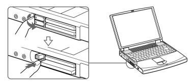
Remove the PC card slot protector.When you use a Type III PC card, you need to remove both the top and bottom PC card slot protectors.
